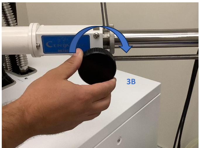
Rotate clockwise to insert detector
